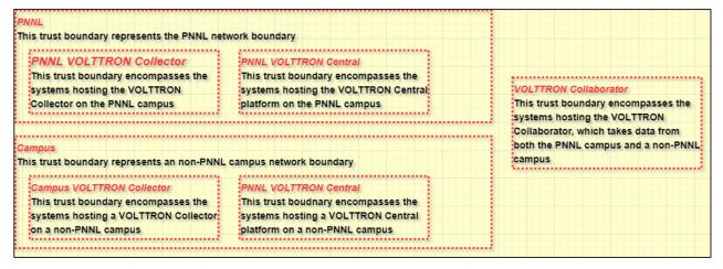
Figure 4. Trust boundaries for VOLTTRON intercampus deployment.
