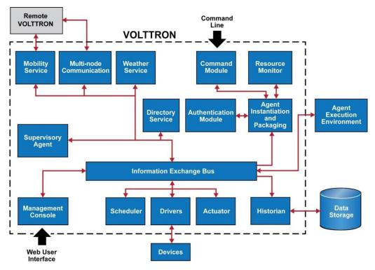
Figure 1. VOLTTRON Platform
